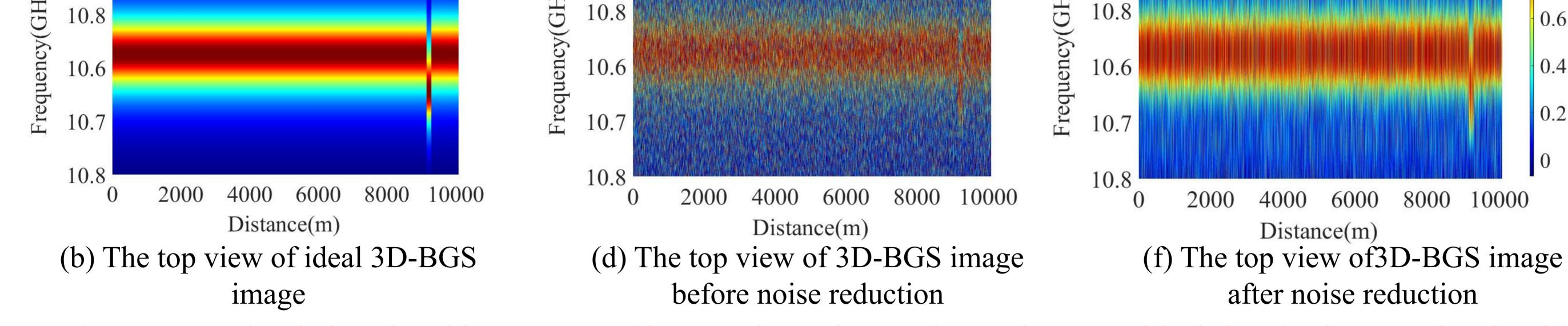
The BOTDR simulation signal is constructed by superimposing random noise on an ideal signal. Then use the algorithm to process the simulated signal to verify the performance of the algorithm.
