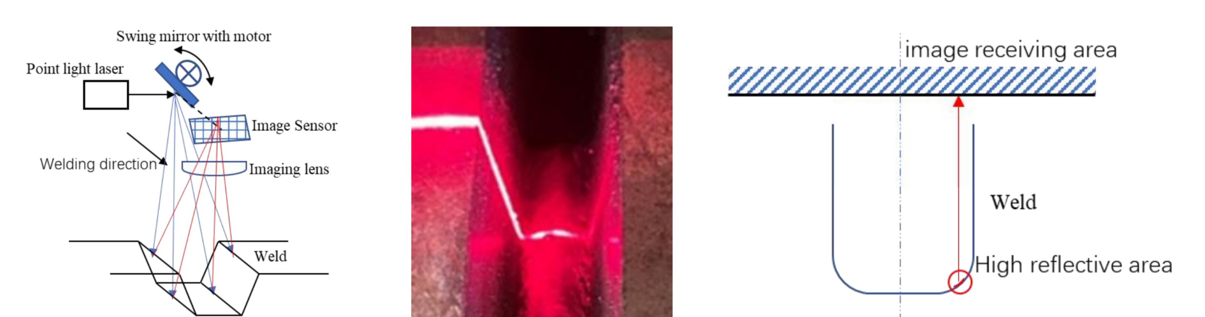
Point-like laser reflection based on Swing Mirror Higher laser brightness, higher signal-to-noise ratio
